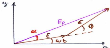
$$\begin{aligned} E_p^2 &= E_1^2 + E_2^2 + 2E_1E_2 \cos \phi \\ &= 2E^2(1 + \cos \phi) \\ &= 4E^2 \cos^2 \frac{\phi}{2} \Rightarrow E_p = 2E |\cos \frac{\phi}{2}| \end{aligned}$$
