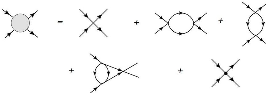
Figure 21.2: The diagrams contributing to the four-point amplitude. The leading order, i.e.  $\mathcal{O}(\lambda)$  diagram is followed by the three possible  $\mathcal{O}(\lambda^2)$  1PI diagrams. The last diagram is the counterterm  $\delta\lambda$ .
