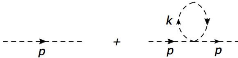
Figure 19.1: 1PI diagrams contributing to the two-point function in the theory with lagrangian (19.1), to order \lambda .
